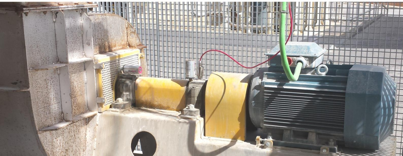
*wise monitoring* online vibration monitoring system allows the user to prevent malfunction of manufacturing equipment. When performance deviates from acceptable operation conditions, the system manages warnings and alarms with EtherNet interface and digital outputs.
